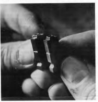
A comparison of the newly-cast type with the original shows that the new sort will "answer tolerably well." Of course, there is an inevitable degradation that must occur in the process, and continued use of the matrix and of the
